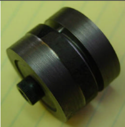
Fixture with rings ready to heat treat
