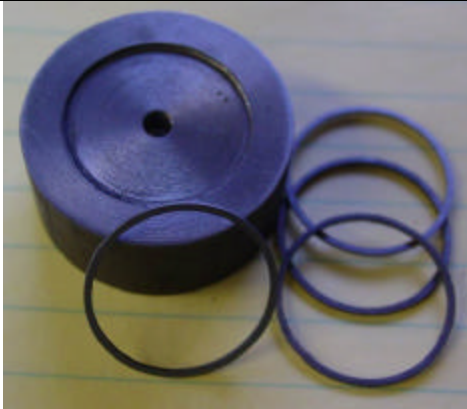
Ring Holder for sanding to thickness
