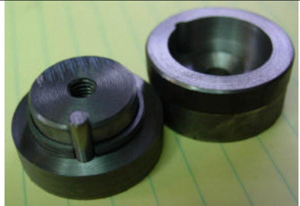
Rings on heat treating fixture
