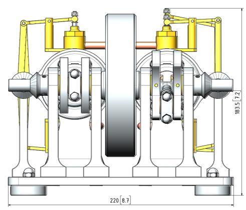
EXP. DUPLEX COMPOUND STEAM ENGINE WITH INDIVIDUAL INLET & EXHAUST VALVES
