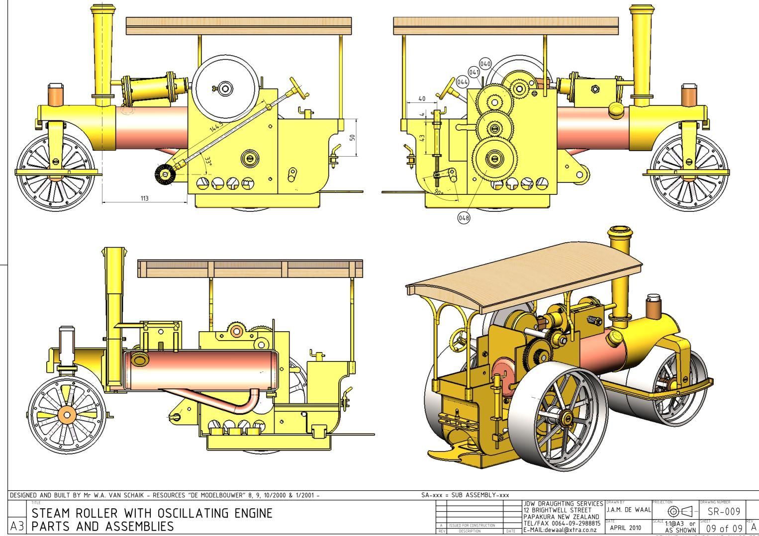
STEAM ROLLER WITH OSCILLATING ENGINE PARTS AND ASSEMBLIES IF NOT STATED ALL CHAMFERS AND FILLETS 0.25mm
